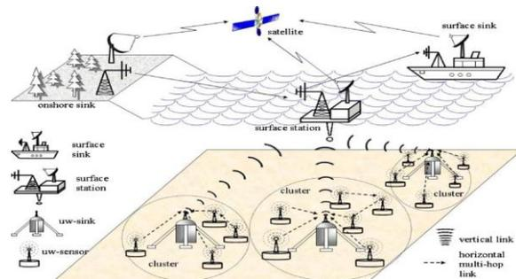
Figure 1. Architecture for 2D underwater sensor networks. [1]
