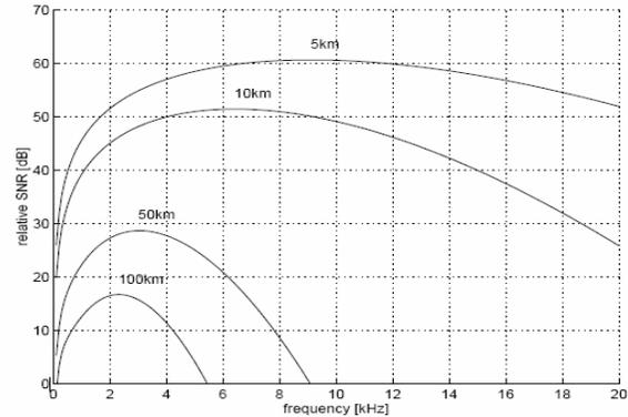
Figure 3. SNR vs. frequency and range for undersea. [11]
