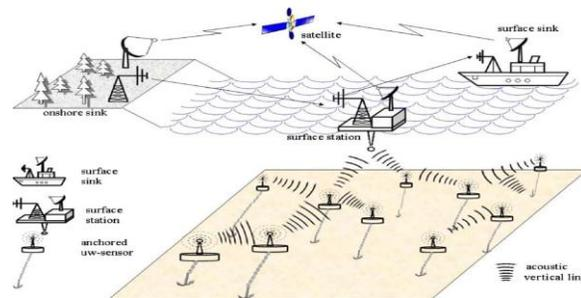
Figure 2. Architecture for 3D underwater sensor networks.[1]
