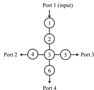
Figure 2. The triplexer formed by 6 coupled resonators
