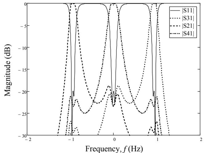
Figure 5. The triplexer response in the normalized frequency.
