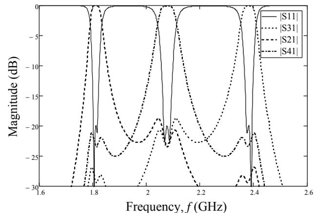
Figure 6. The triplexer response in the denormalized frequency.
