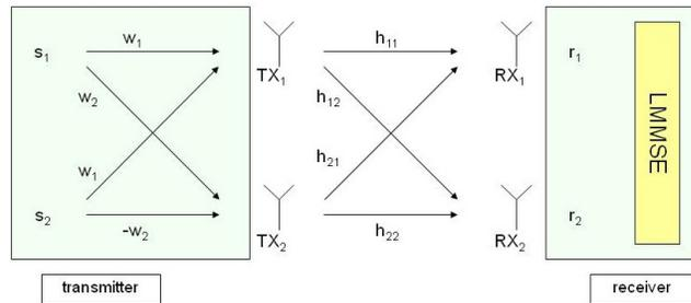
Figure 1. MIMO dual layer transmission, schematic overview.
