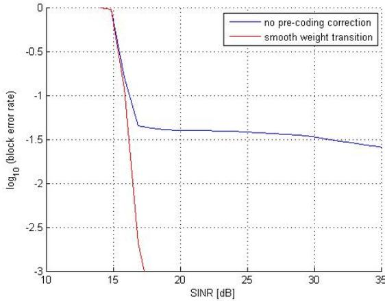
Figure 5. Performance improvement of MIMO Single Stream by smooth transition of equalizer weights. The simulation was executed for a Pedestrian A channel at 3km/h, UE category 20 and CQI 30 according table G in [7]
