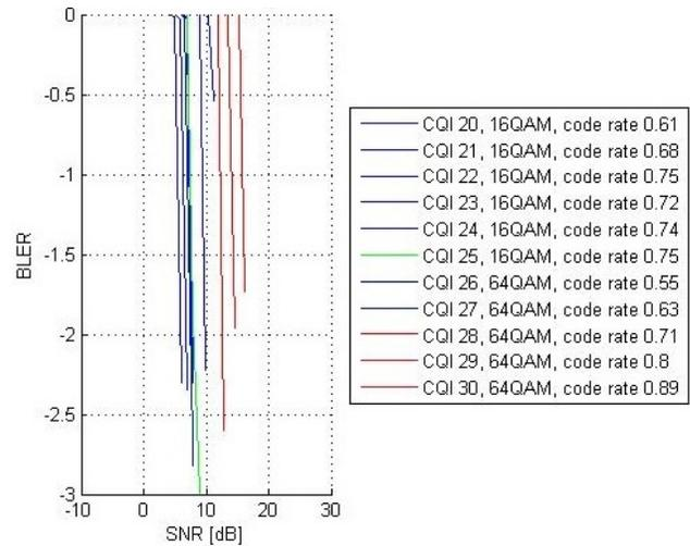
Figure 6. Performance improvement of MIMO Single Stream in AWGN channels by attenuating the changing of the pre-coding vector. The error floor as shown in Fig. 3 can be avoided.
