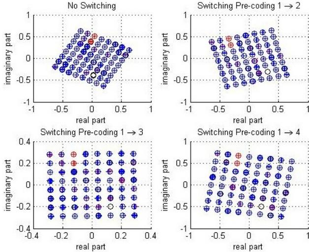
Figure 4. Corrected positions of 64QAM symbols, which are distorted by switching the pre-coding vector in presence of a one tap channel and RRC filter with filter length 20 and OSF 4.
