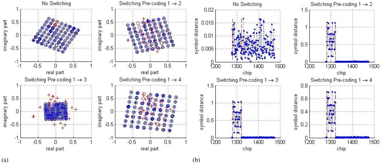
Figure 2. Shifting of 64QAM symbol position due to switching pre-coding vector for a one tap channel and RRC filter with tail length 20. In (a), the expected (o) and measured (+) symbol positions in the complex phase space are shown. In a range around the pre-coding change (red), determined by the maximum channel delay including RC filter, the symbols are distorted. The absolute value of the dislocations as a function of chip index is shown in (b).
