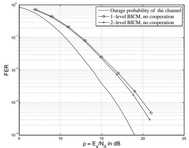
Fig. 7. Frame error rate of the 2-level bit-interleaved coded modulation.
