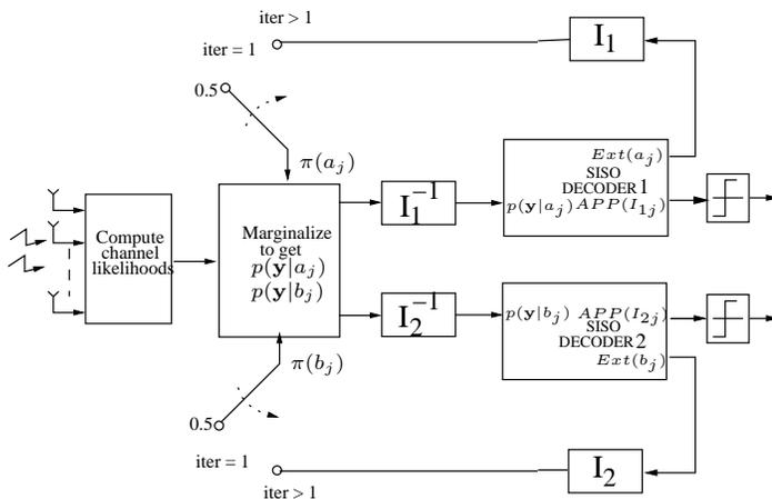
Fig. 4. Two stage iterative MSD decoder.
