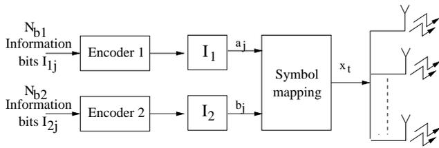
Fig. 1. 2-level BICM transmitter.
