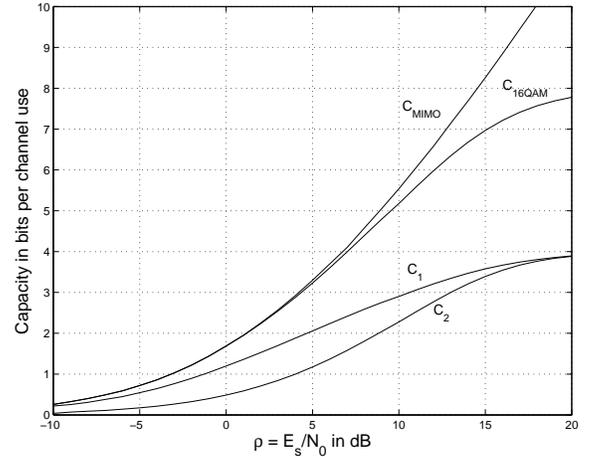
Fig. 3. Capacity of a MIMO channel. 16-QAM constellation.  $n_t = n_r = 2$ .
