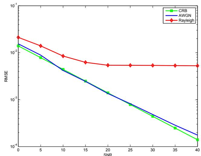
Fig. 5. RMSE of CFO estimator  $\hat{\mu}$  versus SNR (CFO=0.08,  $L = 10$ )
