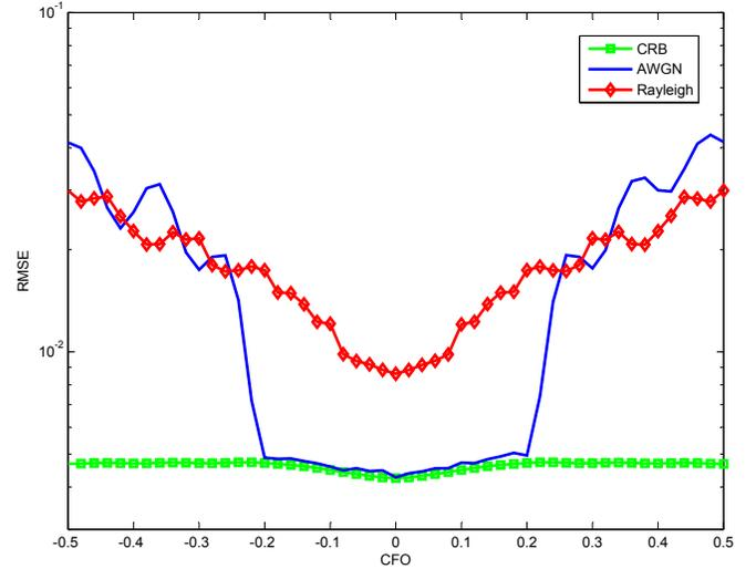
Fig. 3. RMSE of CFO estimator  $\hat{\mu}$  versus  $\mu$  (SNR=10dB,  $L = 10$ )
