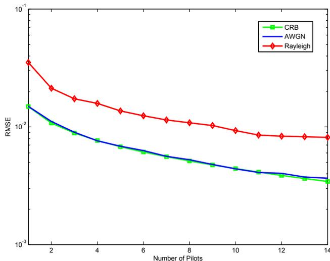
Fig. 4. RMSE of CFO estimator  $\hat{\mu}$  versus  $L$  (SNR=10dB,  $\mu = 0.08$ )
