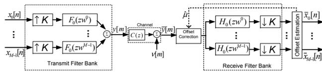
Fig. 1. DFT modulated OPRFB transceiver
