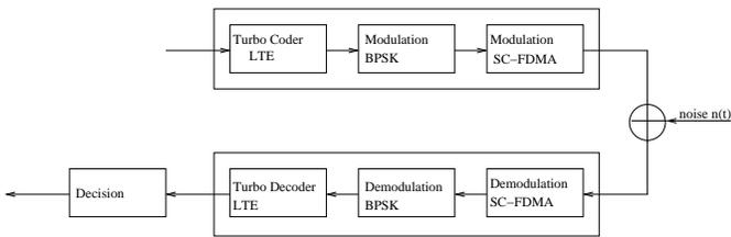
Fig. 1: Coded SC-FDMA System
