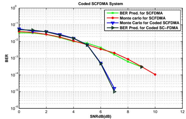
Fig. 7: BER performance comparison for Turbo Coded SC-FDMA
