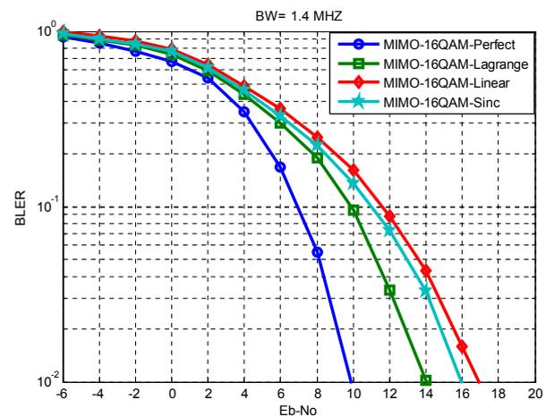
Fig. 6. BLER vs. SNR for MIMO Transmission over Veh-A channel, CQI=7.
