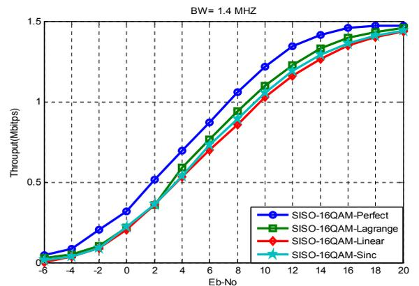
Fig. 7. Throughput vs. SNR for SISO Transmission over Veh-A channel, CQI=7.
