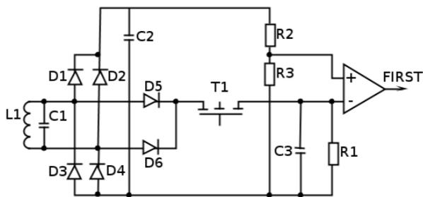
Figure 6. Schematic of the clock & reset building block.
