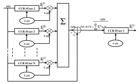
Figure 3. Schematic of the PIC receiver
