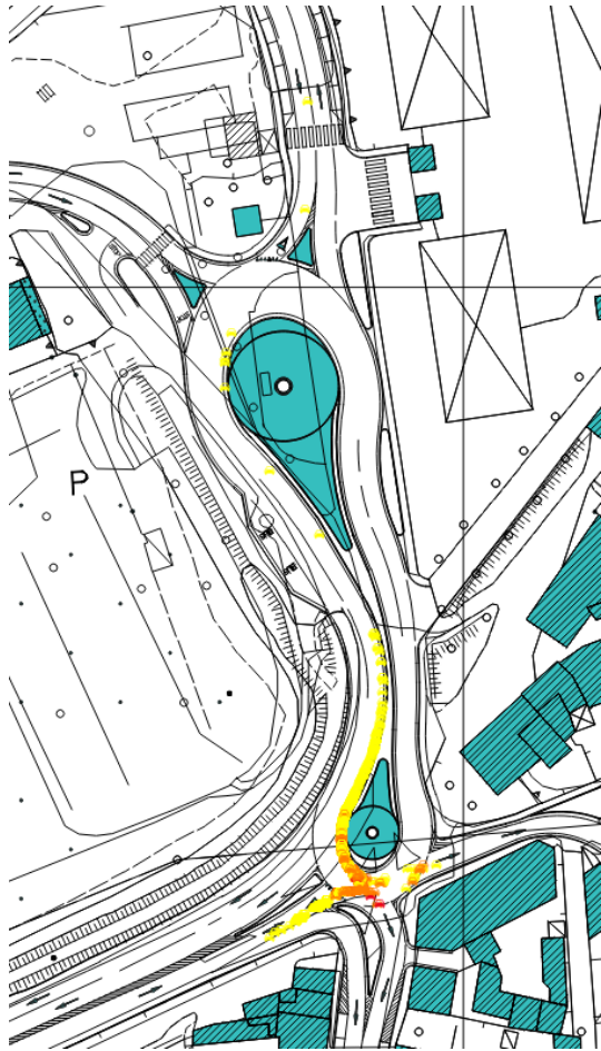
Figure 15. Number of Conflicts obtained by SSAM software and reported on QGIS of the Unconventional Roundabout ("Project Solution")
