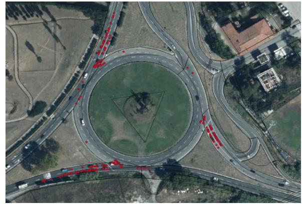
Figure 6. Number of Conflicts obtained by SSAM software and reported on QGIS of 2 nd Unconventional Roundabout
