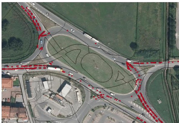
Figure 5. Number of Conflicts obtained by SSAM software and reported on QGIS of 1 st Unconventional Roundabout
