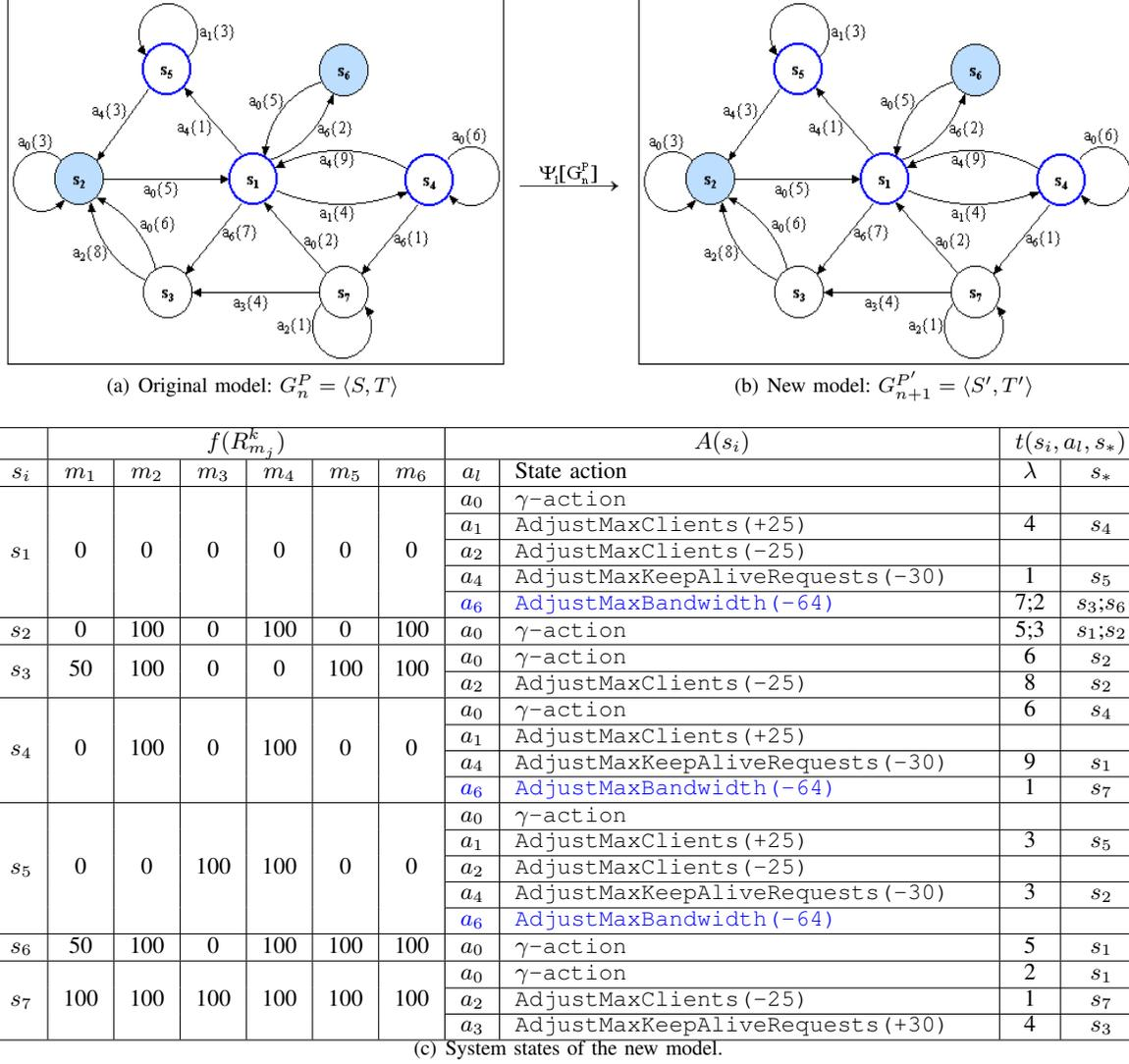
Fig. 5. State-transition model after  $\Delta_{10}[P]$ ; i.e., modifying action  $a_6$  = "AdjustMaxBandwidth(-128)" to "AdjustMaxBandwidth(-64)" in the policies of Figure 1.
