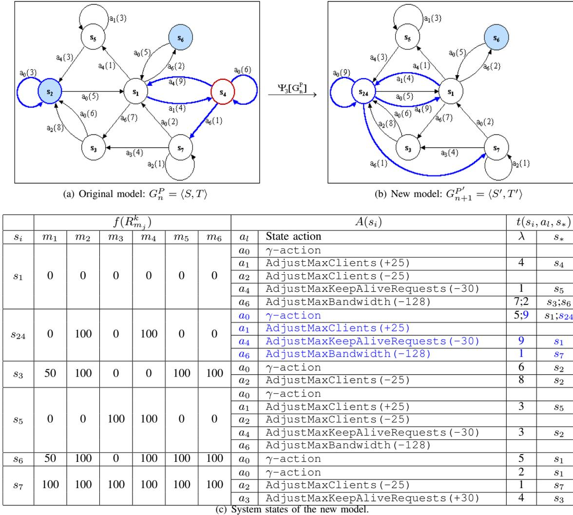
Fig. 7. State-transition model after  $\Delta_7[P]$ ; i.e., modifying the threshold of condition  $c_7 = \text{"APACHE:responseTimeTREND} > 0.0\text{"}$  to  $\text{"APACHE:responseTimeTREND} > -1.0\text{"}$  in the policies of Figure 1.
