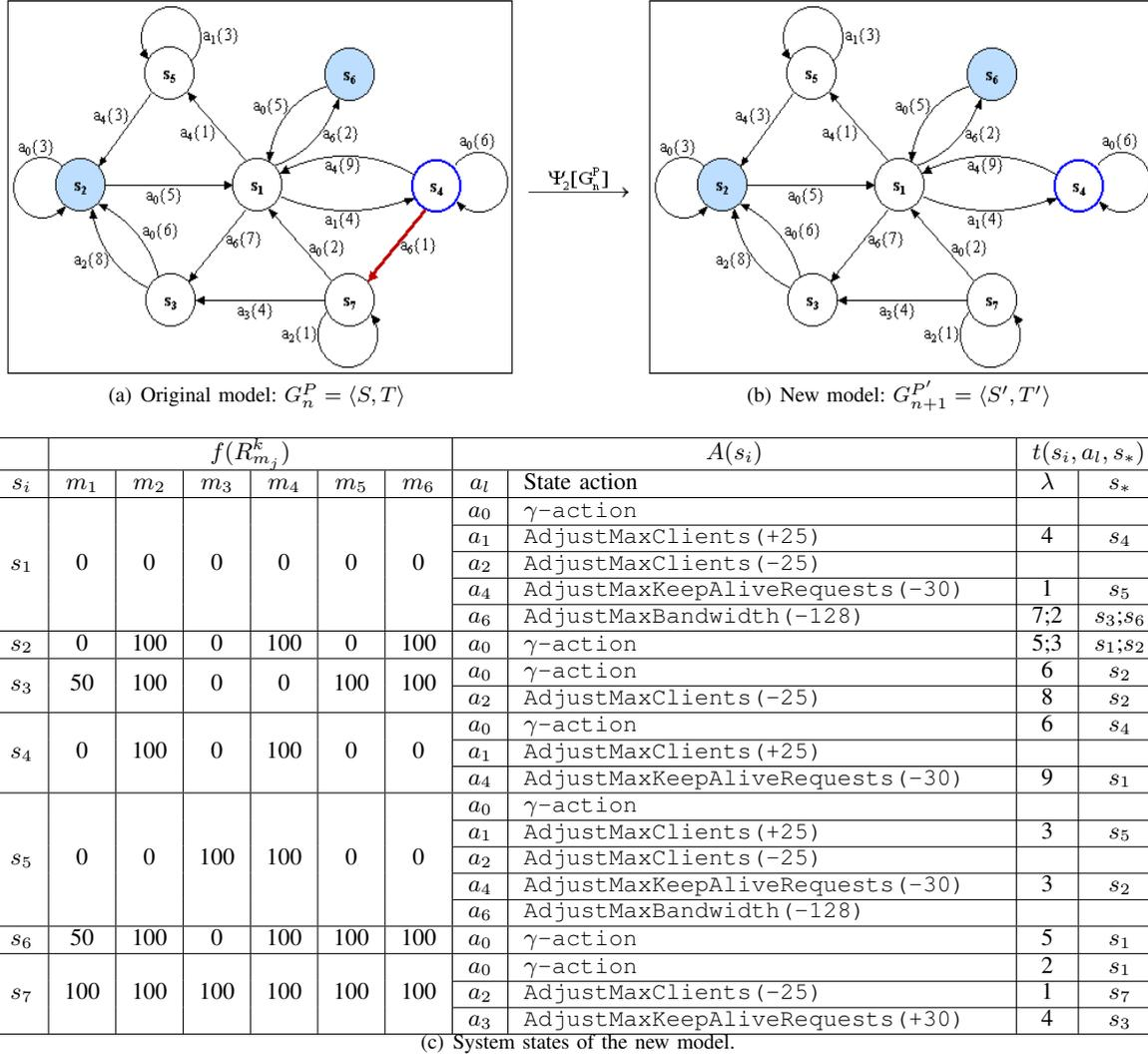
Fig. 6. State-transition model after  $\Delta_9[P]$ ; i.e., removing action  $a_6$  = "AdjustMaxBandwidth (-128)" from policy  $p_2$  in Figure 1.
