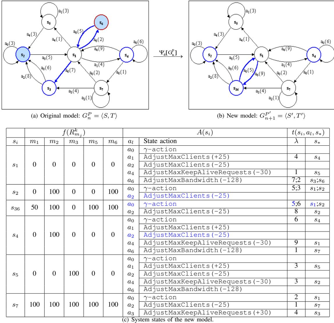
Fig. 8. State-transition model after  $\Delta_4[P]$ ; i.e., deleting condition  $c_5 = \text{"MEMORY:utilizationTREND} > 0.0\text{"}$  from policy  $p_4$  in Figure 1.
