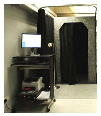
Figure 3. TC<sup>2</sup> whole body scanner (www.itc.polyu.edu.hk).
