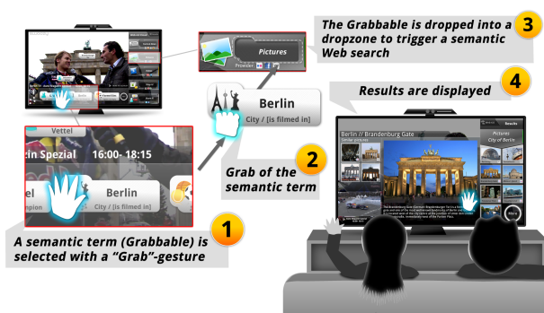
Fig. 13: Grab'n'drop interaction steps to trigger a picture search for the city of Berlin.
