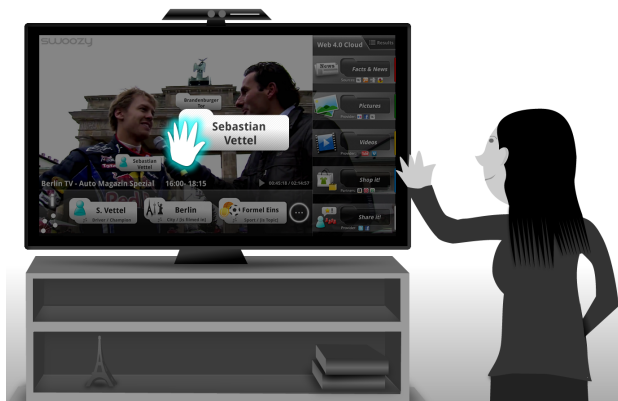
Fig. 12: User gesture interaction: a virtual hand allows the user to grab out a semantic term from a video.
