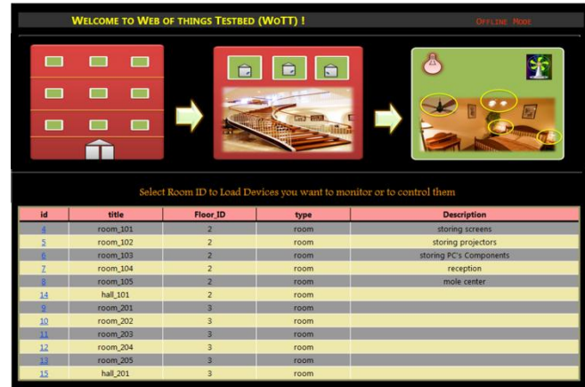
Figure 7. Web pages of virtual gateways get their information from a database server. Sensor Web pages get their information either from direct access to devices or from the offline dataset.
