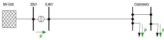
Figure 13. Single line distribution.
