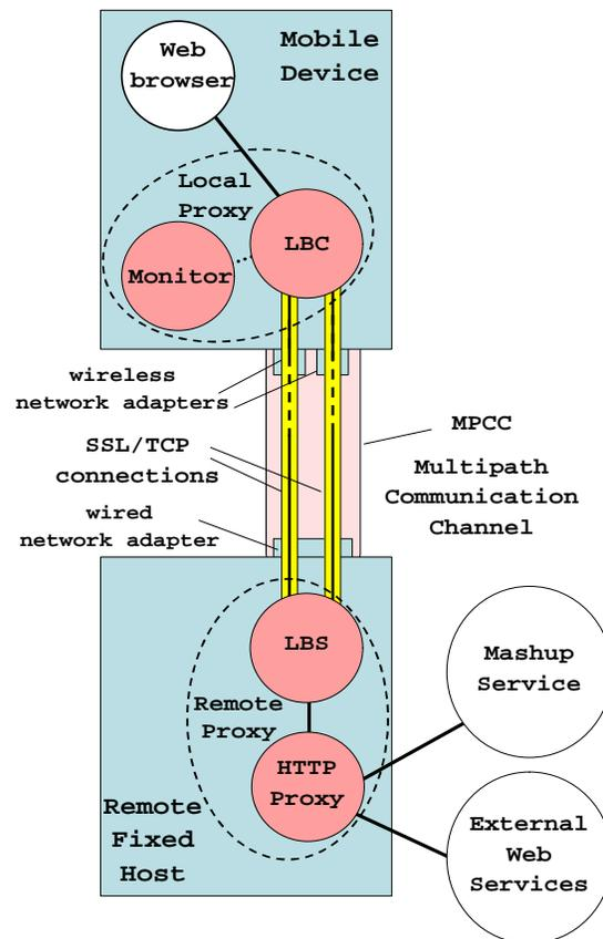
Figure 5: Architecture for Seamless Navigation
