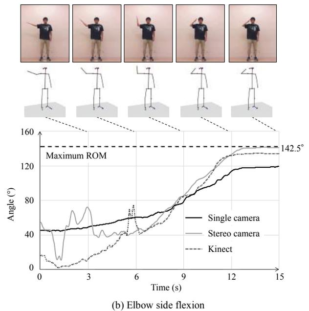
Figure 4. Samples of measurement results with low fluctuations.
