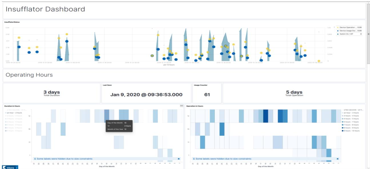
Figure 3. Insufflator dashboard. Key performance indicators of the observed device within a two-month interval
