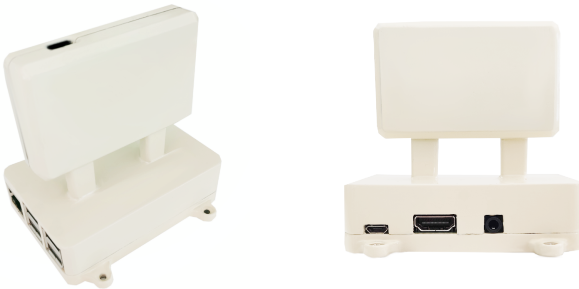
Fig. 2: A prototype of the HealthSonar device. On the left picture, the front side of the device can be seen, while on the right, the back side. The bottom part of the device houses the Raspberry Pi 4 and the top part contains the Aria Sensing LT102 radar module. Various connection ports are located on the top, back, and sides of the device. The radar connects to the Raspberry Pi board via an external USB cable.
