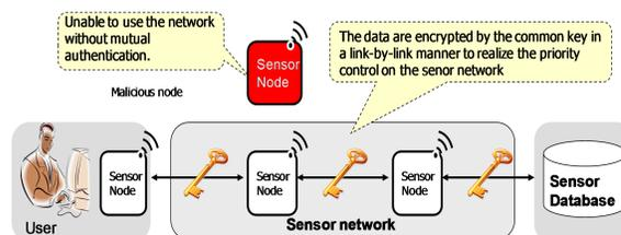
Figure 11. Encryption mechanism of the experimental system
