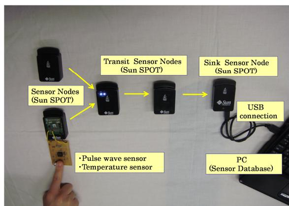
Figure 15. Photo of the experimental sensor network system
