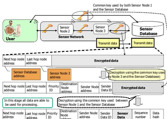
Figure 13. Decryption of the encrypted transmitted sensor data
