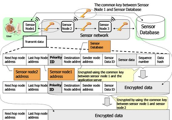
Figure 12. Composition of the transmitted sensor data
