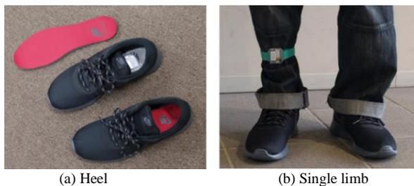
Figure 12. WD attaching position
