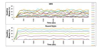
Fig. 10. Twelve H.263 decoders with incremental workload: deadline misses over time
