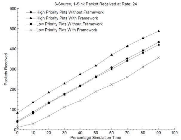
Figure 15. Packets Received for 3 Sources over Simulation Time
