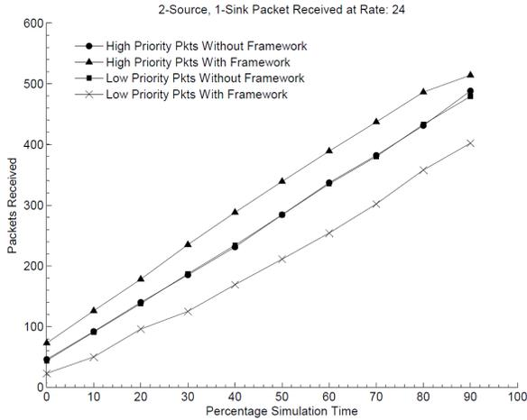
Figure 11. Packets Received for 2 Sources over Simulation Time
