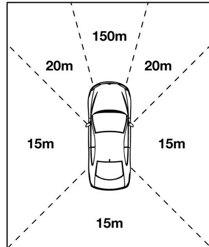
Figure 1. Range and layout of RoadLab cameras
