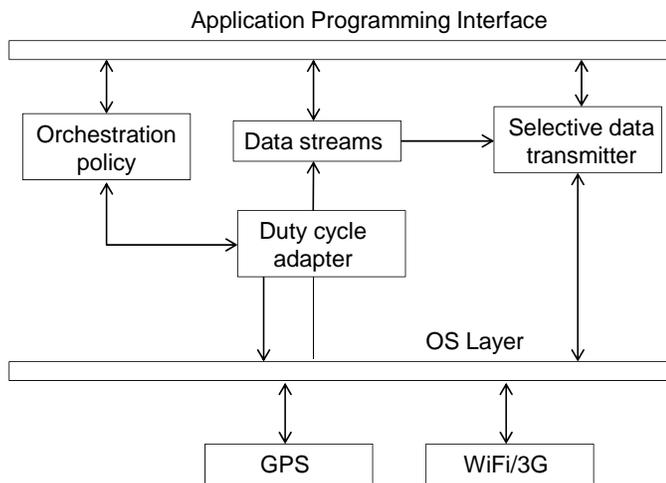
Figure 4. Block diagram of the client software architecture
