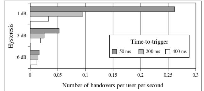
Fig. 5. Simulation results with UE speed of 30 kmph and sliding window size  $T_f$  of 200 ms.
