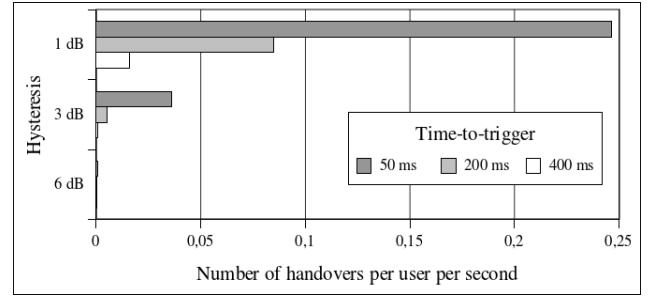
Fig. 4. Simulation results with UE speed of 3 kmph and sliding window size  $T_f$  of 200 ms.
