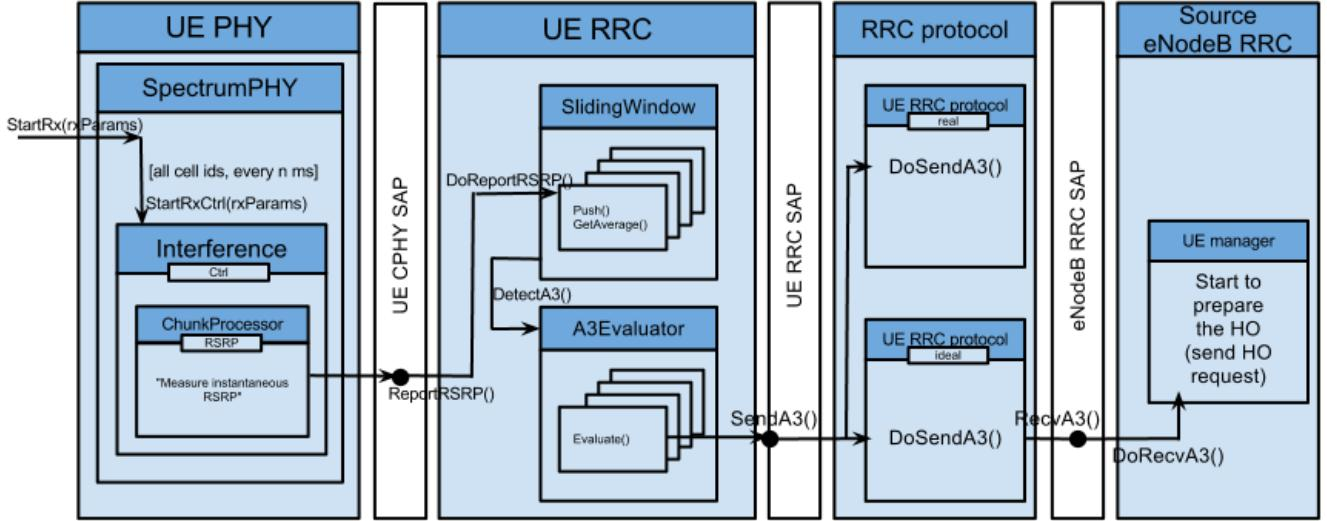
Fig. 2. Implementation of measurements and handover model.
