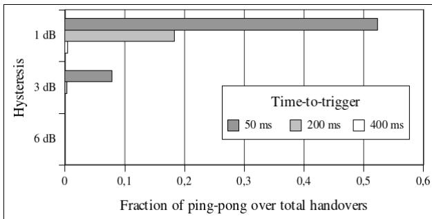
Fig. 6. Rate of ping-pong handovers in simulations with UE speed of 30 kmph and sliding window size  $T_f$  of 200 ms.
