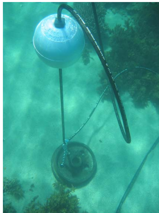
Figure 2 (b): Underwater photograph of the inner mooring with temperature sensors inside the hydraulic cable. Visible in this photograph is the sub-surface float and the wagon wheel anchor. The cable connecting sub-surface float to the surface buoy is floating loose to allow tidal variations.
