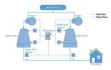
Figure 1. Water distribution plant tested architecture
