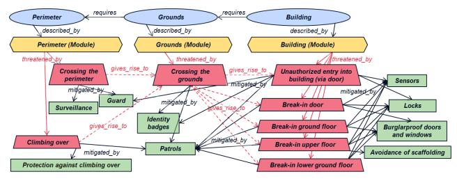
Figure 4. Graph model for the physical environment scenario (excerpt).
