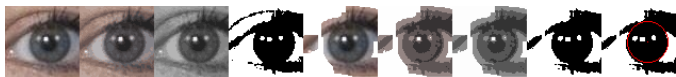
Figure 4. Circle detection on an eye of a real person using the London Face Set [18].
