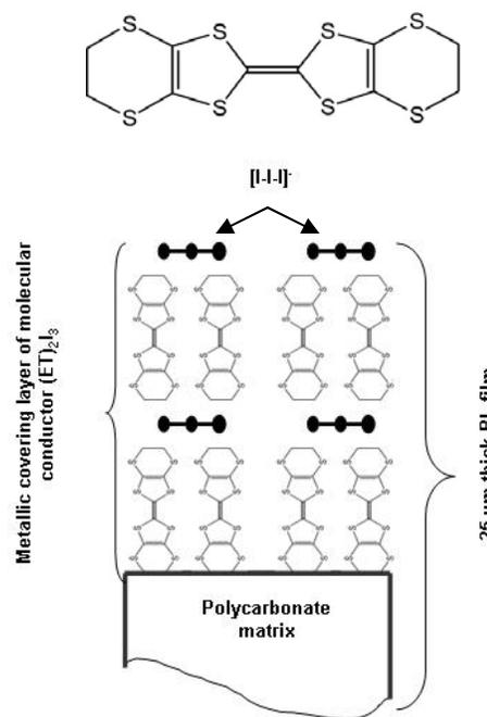
Figure 1. Top: Skeletal formula of bis(ethylenedithio)tetrathiafulvalene (ET); bottom: schematic view of the orientation of (ET)<sup>+0.5</sup> radical cations and [I-I]<sup>-</sup> anions in a metallic covering layer of  $\beta$ -(ET)<sub>2</sub>I<sub>3</sub> formed at the surface of a polycarbonate film.
