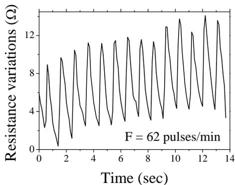
Figure 4. Resistance response to the blood-pulse movement.
