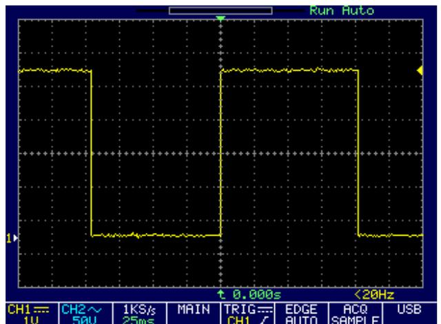
Figure 8. Oscillograms of minimal frequency signal (~ 5 Hz).
