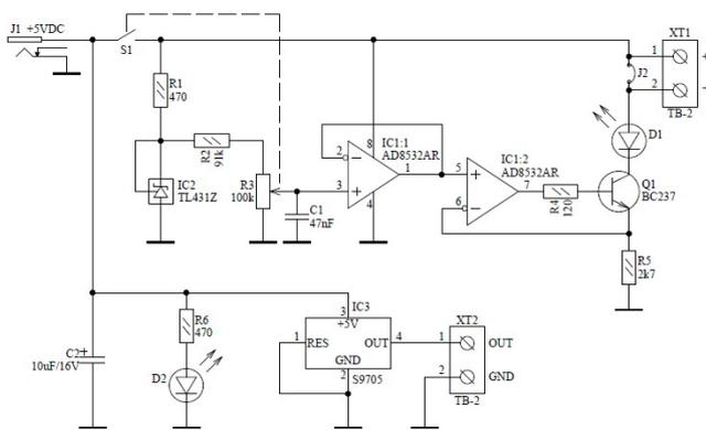
Figure 5. Circuit diagram of LED evaluation board.
