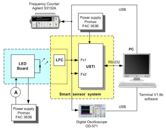
Figure 4. Measuring set-up.
