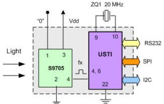
Figure 2. Circuit diagram of optoelectronic sensor system.
