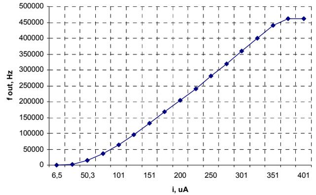
Figure 13. Output frequency vs. current through a white light diode.
