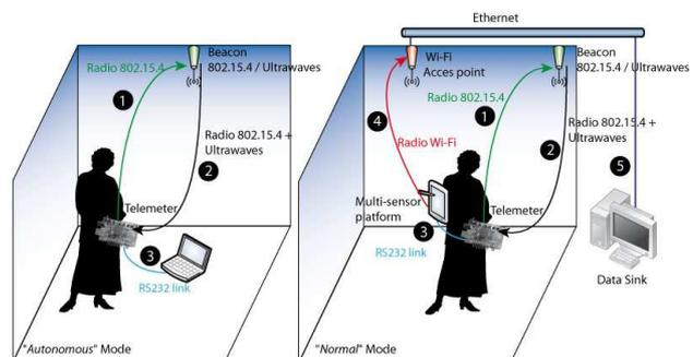
Figure 1. System architecture and two possible modes.
