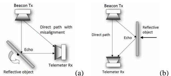
Figure 12. Test configurations for evaluating multipath effects.
