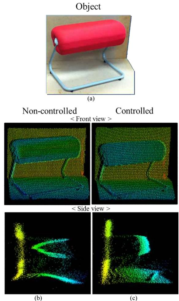
Figure 6. (a) A measured object (b) the non-controlled scanning result (c) the controlled scanning result
