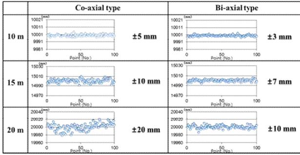
Figure 3. Distance accuracy according to optical system types
