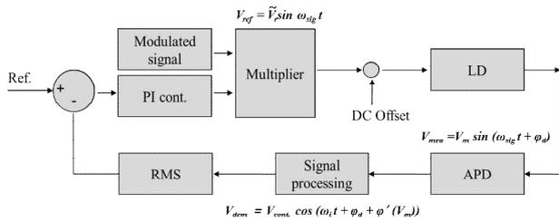
Figure 5. A block diagram of the intensity control method
