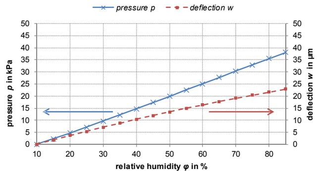
Fig. 7. Influence of the relative humidity on the deflection of a  $20 \mu\text{m}$  silicon flexure plate coated with a PVA/PAA hydrogel blend for the BIZEPS™ sensor of type A based on the bimorph effect.
