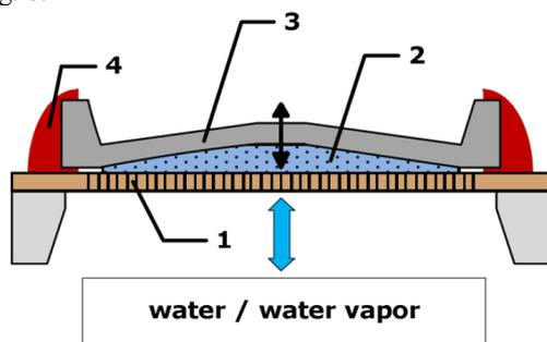
Fig. 6. BIZEPS™ sensor switch based on volume swelling (type B): 1. porous  $\text{Al}_2\text{O}_3$  membran, 2. crosslinked PVA/PAA layer, 3. silicon chip with a  $20 \mu\text{m}$  silicon flexure plate, 4. silicone glue Scrintec® 901.
