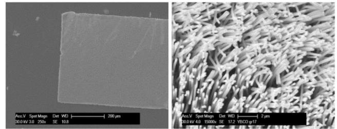
Fig. 4. SEM image (left with low, right with high magnification) of gold nanowires with a density of about  $1/\mu\text{m}^2$ , 200 nm diameter, 10  $\mu\text{m}$  length and an aspect ratio of 90:1 [5].
