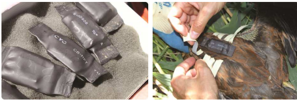
Figure 9. Left—Photo of devices ready to be used; “encapsulated” using two layers of thermo-contractile sleeve in opposite directions and in between a layer of silicone. Right—Test with cranes; placement of a tracking device.
