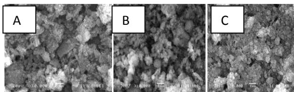
Figure 1. SEM micrographs for (A) Native HAp, (B) 0.5wt% CNT blended HAp, (C) 0.7wt% CNT blended HAp showing variations in surface topography due to the presence of CNT.
