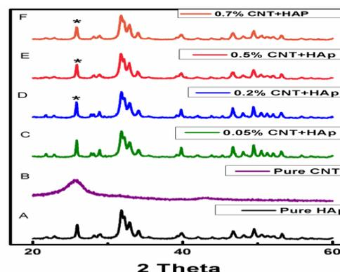
Figure 2. X-ray diffraction pattern of native HAp, CNT and CNT blended HAp material (\* represents the peak for CNT): Y-axis has arbitrary units.
