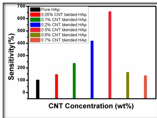
Figure 5. Variation in sensitivity for different CNT concentrations in HAp, at room temperature (30 °C) for 100 ppm methanol
