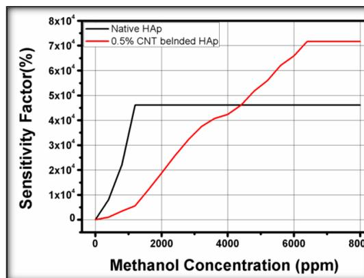
Figure 7. Sensitivity of native HAp and 0.5% CNT blended HAp thick films for various concentrations of methanol vapours at room temperature (30°C).
