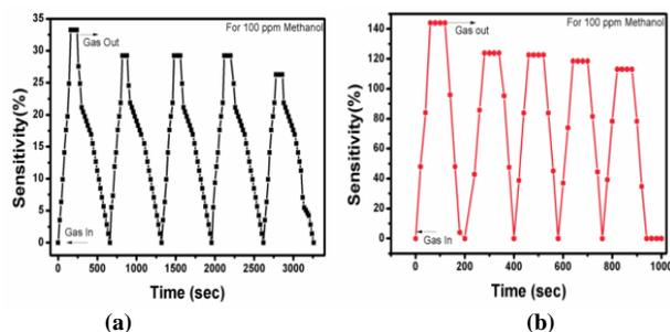
Figure 6. Response/ recovery time plot for native HAp and 0.5wt% CNT blended HAp thick film in the presence of 100 ppm methanol. Continuous repeated cycles for response / recovery time at room temperature (30 °C), (a) native HAp, (b) 0.5% CNT blended HAp.
