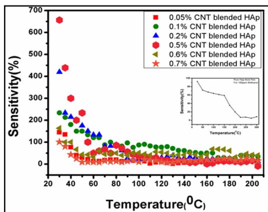
Figure 4(A). Sensor sensitivity (response) of native HAp and CNT blended HAp at variable temperature for 100 ppm concentration of methanol
