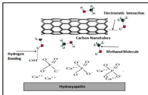
Figure 4(B). Formation of hydrogen bonding, due to dipole- dipole interaction between polar methanol molecule and hydroxyl ions on HAp surface. Electrostatic interaction between methanol and CNT molecules leads to enhance the sensing property of the substrate material
