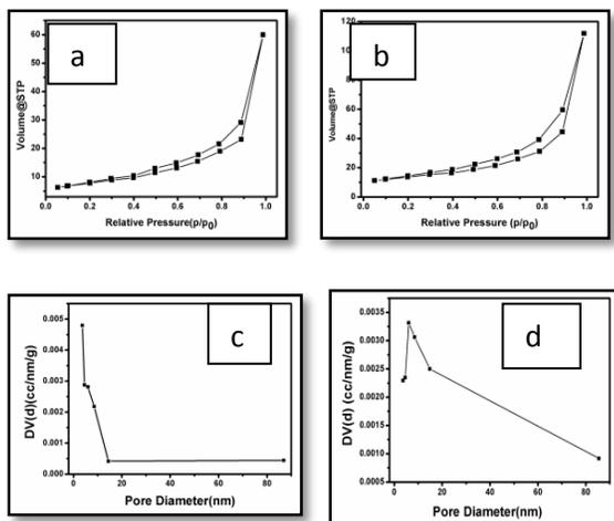
Figure 3. N<sub>2</sub> adsorption/desorption isotherm (a) native HAp, (b) 0.5wt% CNT blended HAp and BJH pore size distribution curve (c) native HAp, (d) 0.5wt% CNT blended HAp.
