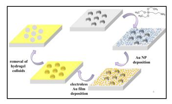
Figure 1. Major steps involved in the fabrication of sub-wavelength holes in gold films.
