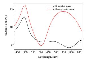
Figure 5. Transmission spectra of a sensor before and after coating with gelatin.
