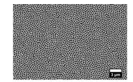
Figure 2. Representative SEM image of a prepared periodic hole array in a metallic film.
