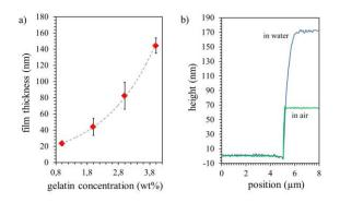
Figure 4. Gelatin films on sensor surface. a) gelatin film thickness in dependence of the gelatin concentration in the soultion used for spincoating. b) Gelatin film thickness in air and in water determined using atomic force microscopy (AFM).
