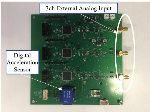
Figure 5. Sensor board.
