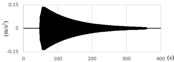
Figure 8. Input swept sine wave (2 to 20 Hz).
