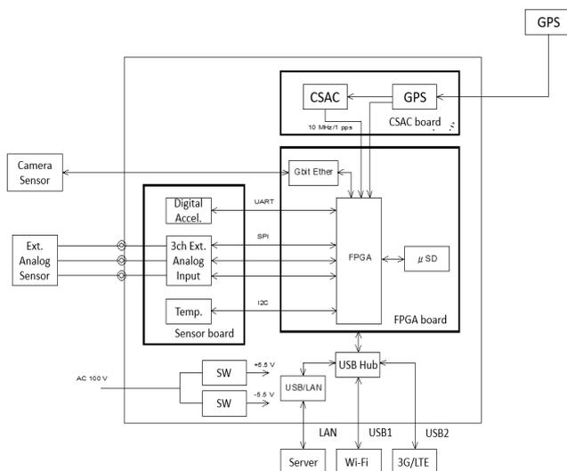
Figure 1. Configuration of digital sensing platform.
