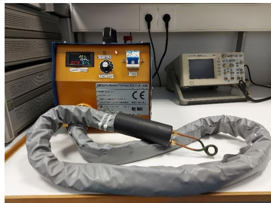
Figure 9. RF heater for localized stress annihilation
