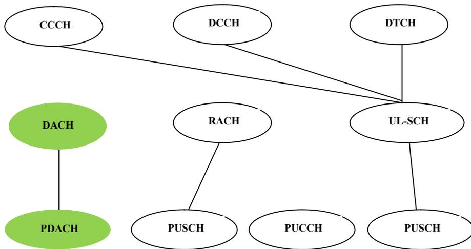
Figure 5. The uplink channel architecture for the OMC.
