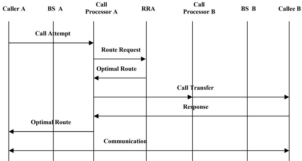
Figure 4. An example of a call processing flow of OMC.
