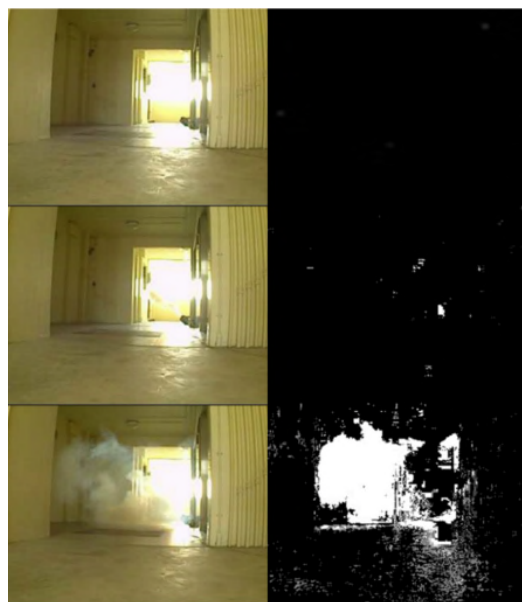
Figure 4. Background Substraction using GMM [1]
