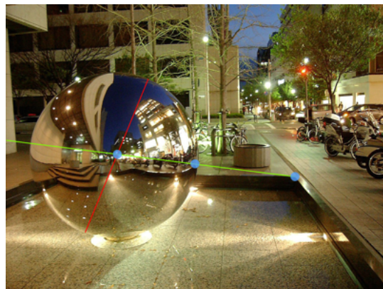
Figure 4. Finding the sphere's center from a single pair of corresponding points and the major axis of the ellipse. The green line connects the corresponding points, while the red line represents the major axis of the ellipse.
