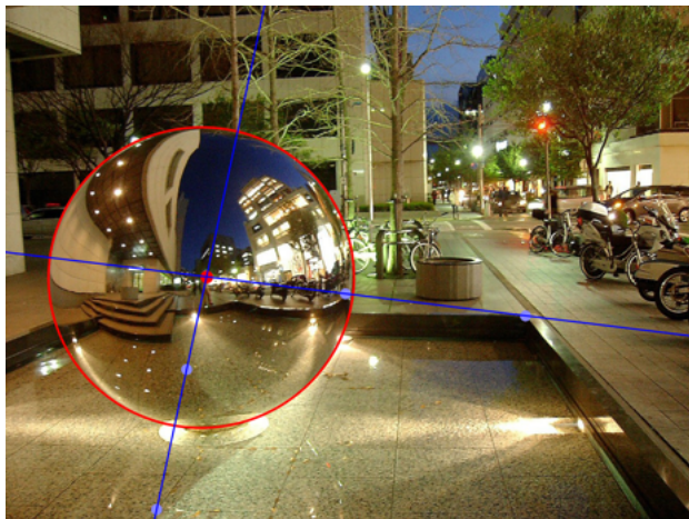
(b) Finding the sphere's center in the image from two pairs of corresponding points.
