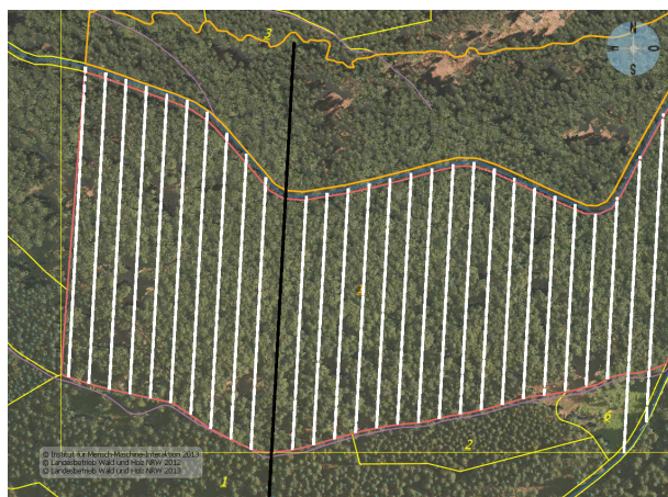
(a) 20 m distance between adjacent skidding roads.
