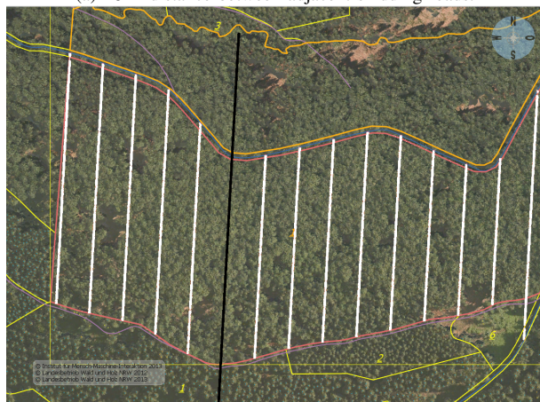
(b) 40 m distance between adjacent skidding roads.
