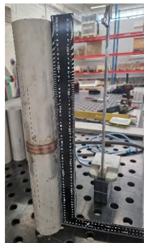
Figure 11. Straightness in pipe after welding.
