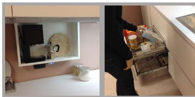
Figure 4. Electromechanical systems: the wall unit device (on the left), the system for base cabinet (on the right).
