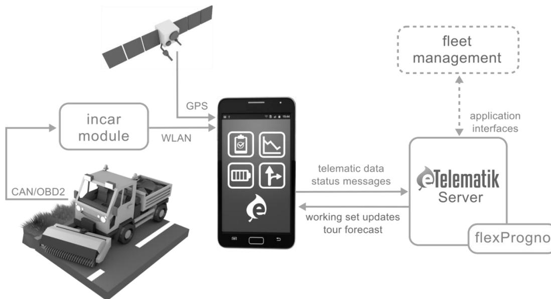
Figure 1. eTelematik system architecture overview (adapted figure, based on original by Johannes Kretschmar, University Jena)
