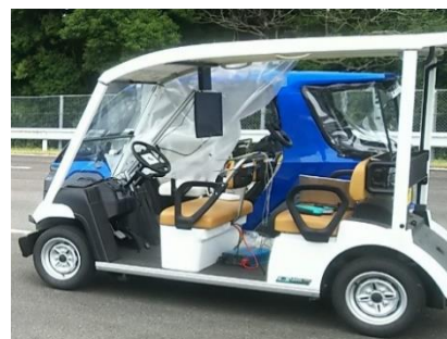
Figure 9. The vehicle with remote type automated system
