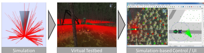
Figure 2. Difference between a simulation (of a single laser scanner), a Virtual Testbed (of a laser scanner equipped wood harvester and its operational environment) and Simulation-based X (user interface of a Simulation-based Control approach).
