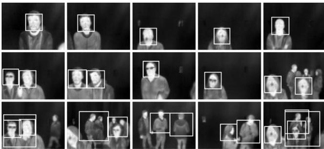
Figure 22. Examples of the detection using Haar Cascade algorithm with the improved classifier for thermal images.
