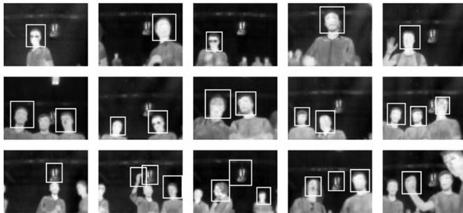
Figure 32. Examples of the face detection using Chamfer Matching algorithm.
